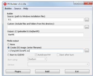
fig. 6: PE Builder configuration dialog
